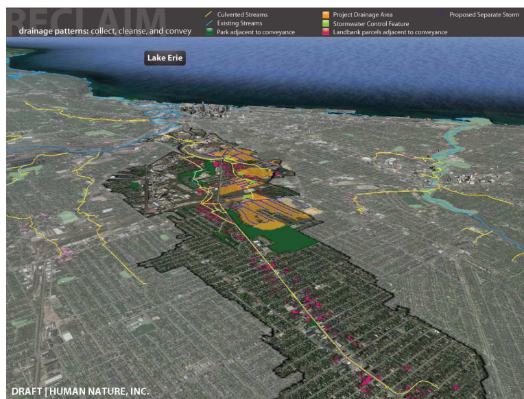
NEORSD analysis of potential sites along culverted streams (Draft). Printed with permission from the NEORSD. Image credit: Human Nature & Strand Associates
