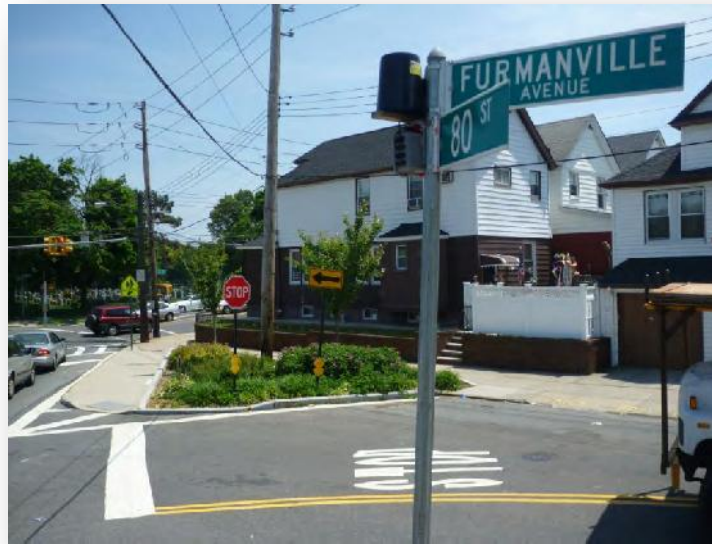
Figure 6. Rain gauge installed on street sign as part of monitoring program. Photo credit: Drexel University, Kimberly DiGiovanni June 2010.
