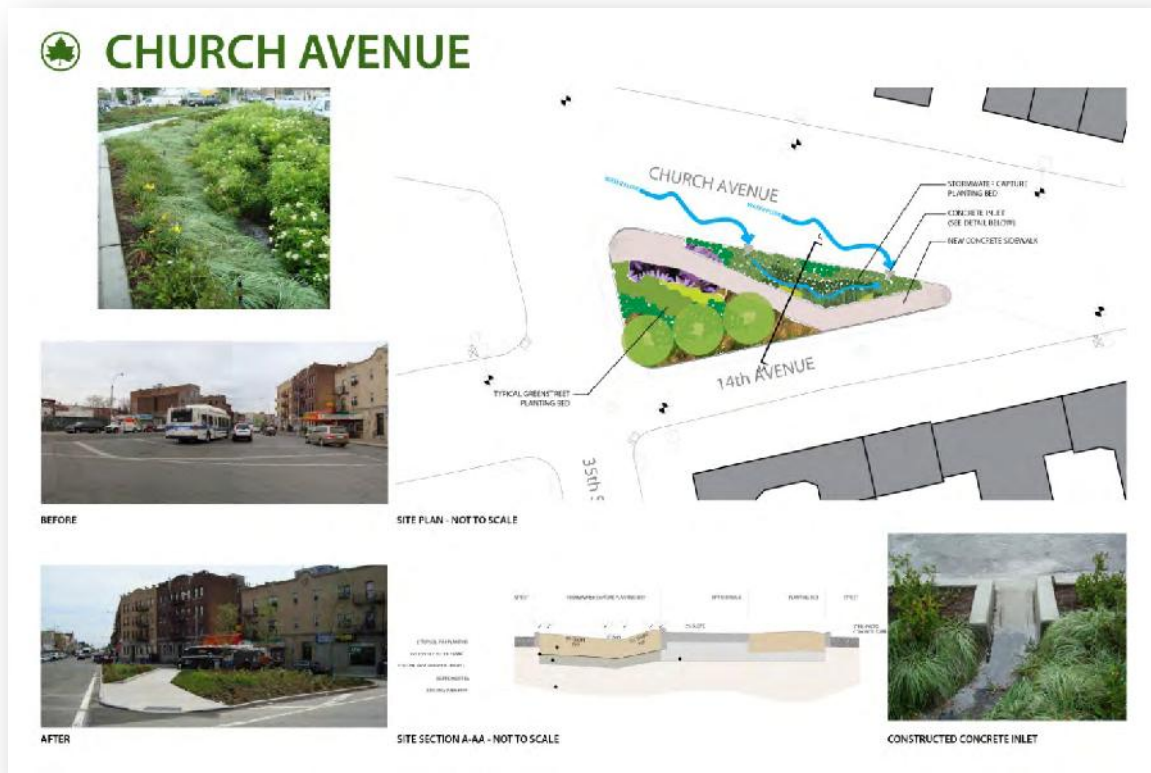
Figure 3. Church Avenue site plan that shows before and after renderings, conceptual landscaping and water flow (site plan), cross section of bioretention area (site section A-AA).
