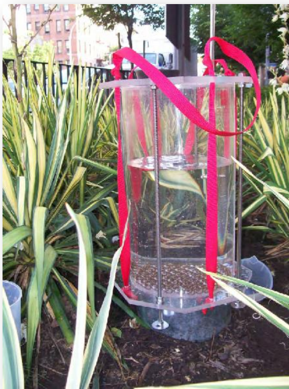
Figure 4. Infiltration testing. Photo credit: Drexel University, Kimberly DiGiovanni June 2010.
