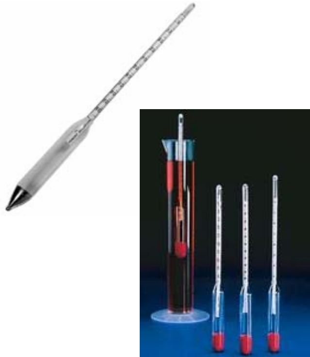
Hydrometers and a Hydrometer Jar holding both a sample liquid and a hydrometer
